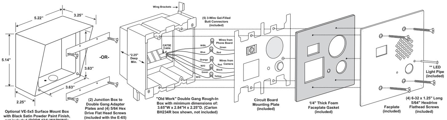
**\* CAUTION:** Excessive wire length and/or using a rough-in box with inadequate depth can apply force to the circuit board causing physical damage.
