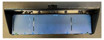
Place the corresponding smokes acrylic lens (be sure to remove protective lens) over the circuit board
