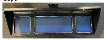
Reinstall the factory bezel using the original mounting hardware.
