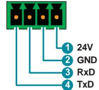
*Note: The 24-volt pins (pin 1) are included to provide power to a dedicated external control product and should NOT be used when connecting a standard RS-232 device*
