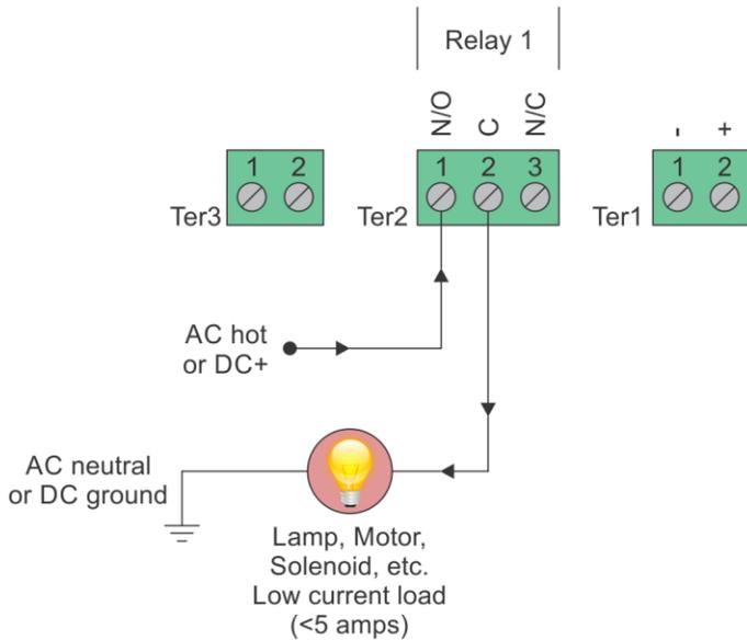
**Internal Relay - Loads Less Than 5 Amps**
