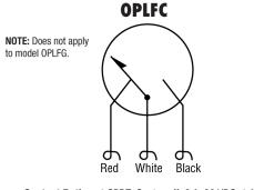
Contact Rating: 1 SPDT; Center off; 2 A, 30 VDC, 1 A, 125 VAC pilot duty
