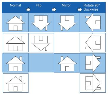
The camera may be installed on a vertical, side-facing, or tilted surface in order to accommodate the interior or exterior design of a building. The interior of a building can be shaped as a narrow rectangular space, such as corridor. The conventional HD image, such as that of a 16:9 aspect ratio, will be incongruous with its wide horizontal view. With video rotation, the camera can more readily cover the field of view on a tall and narrow scene.
