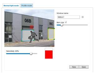
The Percentage Indicator will rise or fall depending on the variation between sequential images. When motions are detected by the Network Camera and are considered to exceed the preset threshold, the red bar rises. Meanwhile, the motion detection window will be outlined in red.
