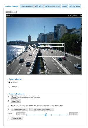
Use the **Media** > **Image** > **Focus** function to tune for a best image focus on your target area. If using a non-iCS lens model (RBF lens), you should manually tune the focus to be close to the optimal, and then use the auto scan focus function.
