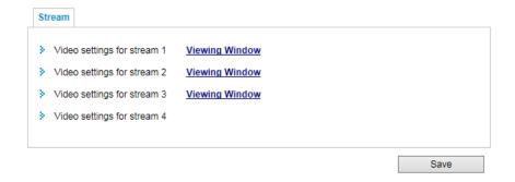
This Network Camera supports multiple streams with frame sizes ranging from 480 x 272 to 1920 x 1080 pixels.
