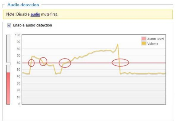
The red circles indicate where the audio alarms can be triggered when breaching or falling below the preset threshold.
