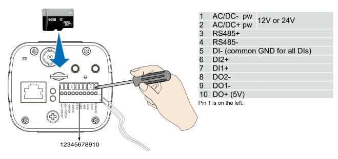
The DO pin can provide a 5V output, and the max. load is 50mA.
