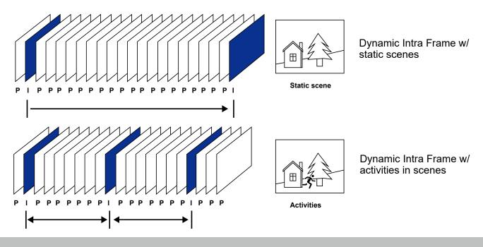
With the H.265 codec in an optimal scenario and when Dynamic Intra frame is combined with the Smart Stream function, an 80% of bandwidth saving can be achieved compared with using H.264 without enabling these bandwidth-saving features.
