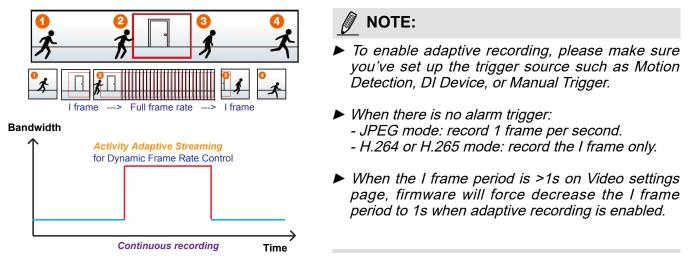
The alarm trigger includes: motion detection and DI detection. Please refer to Event Settings on page 115.
