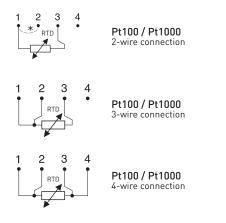
$\ast$  Short terminals 1 and 2 on the transmitter, max 50  $\Omega$  on each wire
