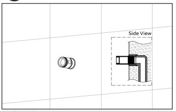
Inlet fitting(4) installed.
