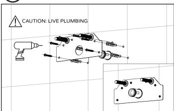
Drill hole previously marked and add anchors(7). Place wall mount plate(5) over the holes and secure with screws(8).
