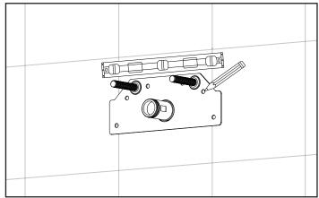
Place wall mount plate(5) over the inlet fitting(4) and make sure it is leveled. Mark holes with pencil.
