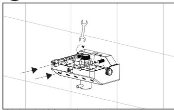
Slide shower body(11) over wall mount plate(5) screws and secure with nut(12).
